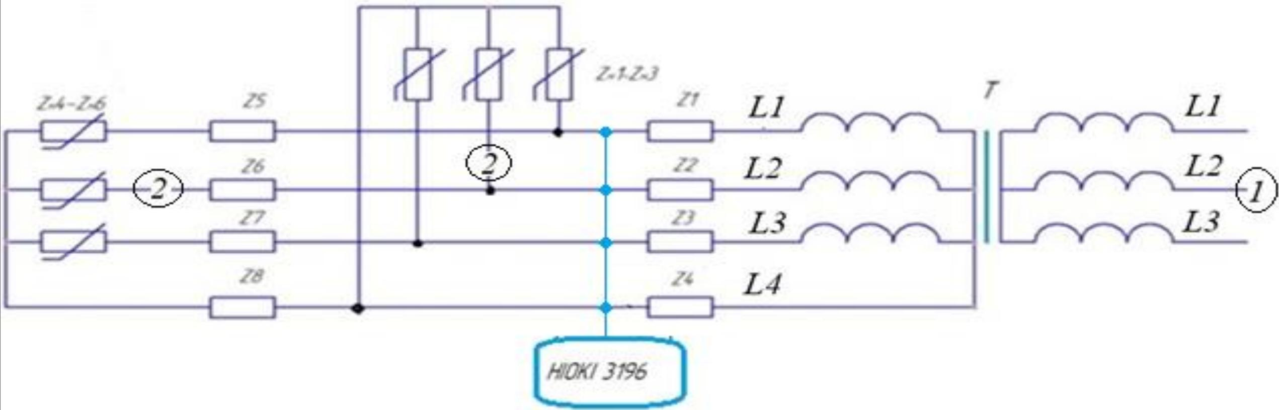
Interest to study the operating modes of a power transformer loaded with a non-linear and asymmetric load, namely under conditions of extreme voltage asymmetry - phase break on the 10 (6) kV voltage side
