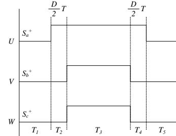
(1) Stator resistance  $R_s$ At the initial stage, DC excitation voltage  $U_a$  is injected into the PMSM, and the current signal  $I_a$  on the PMSM is collected.(2) D-axis inductance  $L_d$  and Q-axis inductance  $L_q$
